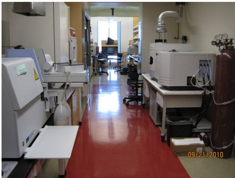
The ICP-AE (right) and graphite furnace AA (left) are part of EALS capabilities for trace metal analyses.
